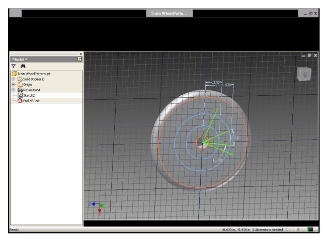
After the wheel is revolved flip the piece over and put a 2D sketch on the back then recreate the lines above and dimension correctly. Then you need to extrude cut the shape out.
