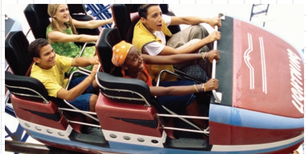
A lap bar restraint lowers and goes across the lap of a seated rider. It prevents a rider from standing up during the ride.
