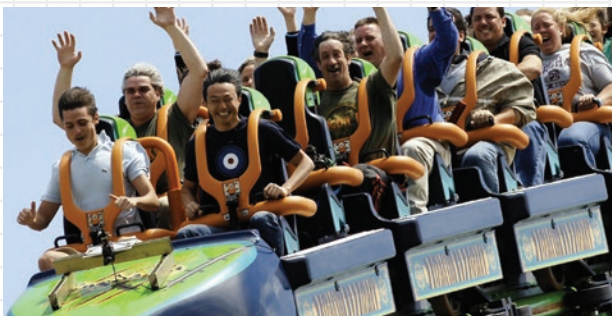
An over-the-shoulder restraint rotates down to fit over the shoulders and sometimes across the chest and waist.
