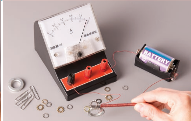
This electromagnet has 60 loops of wire wrapped around its core and can pick up heavier washers.
