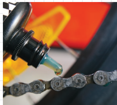
Oil is applied to a bike chain to reduce friction between the chain and gears.
