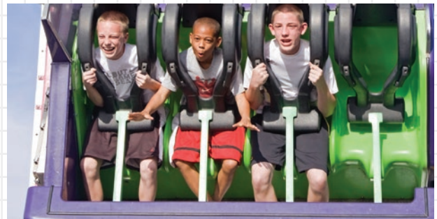
A T-bar rotates toward a rider and locks in place. Here a T-bar restraint combines with an over-the-shoulder restraint.
