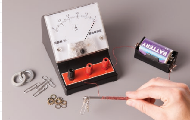
This electromagnet has 30 loops of wire wrapped around its core and can pick up light paper clips.
