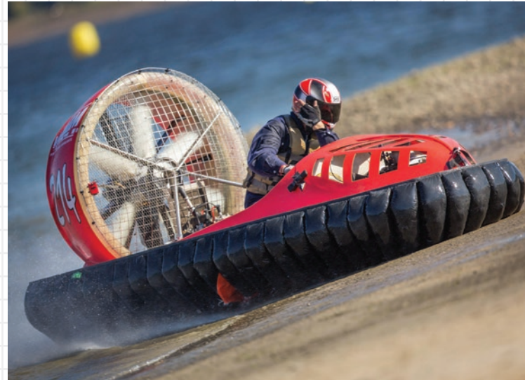
This hovercraft coasts on a thin layer of air over land or water. The propeller on the back of the craft propels the hovercraft forward.
