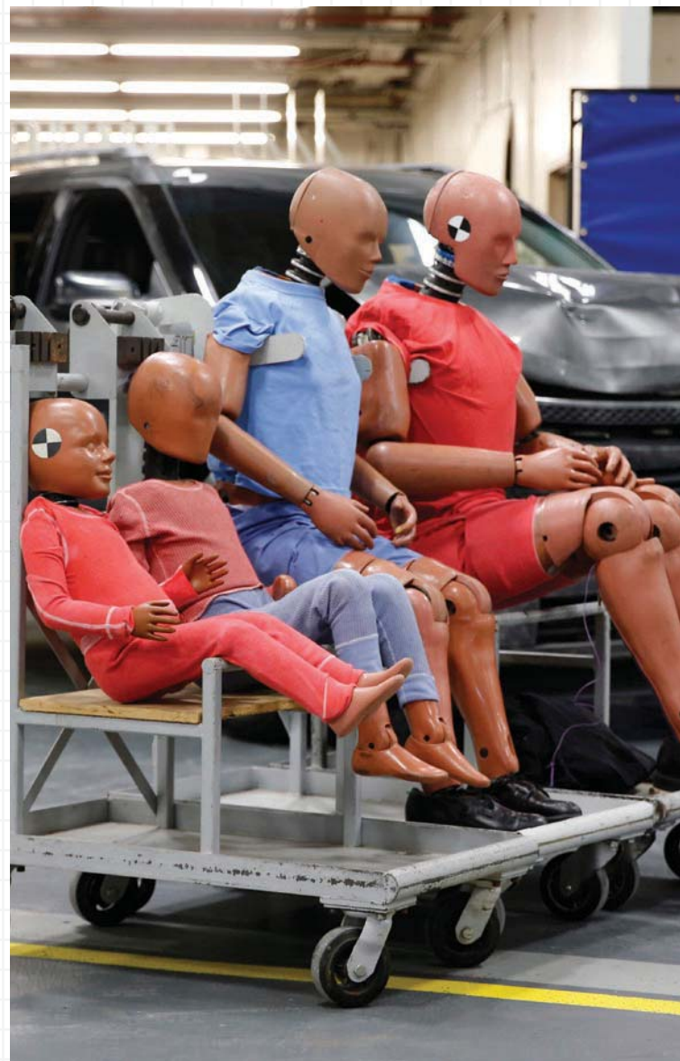
Crash test dummies are used to test how the energy transfers in automobile accidents affect passengers.
