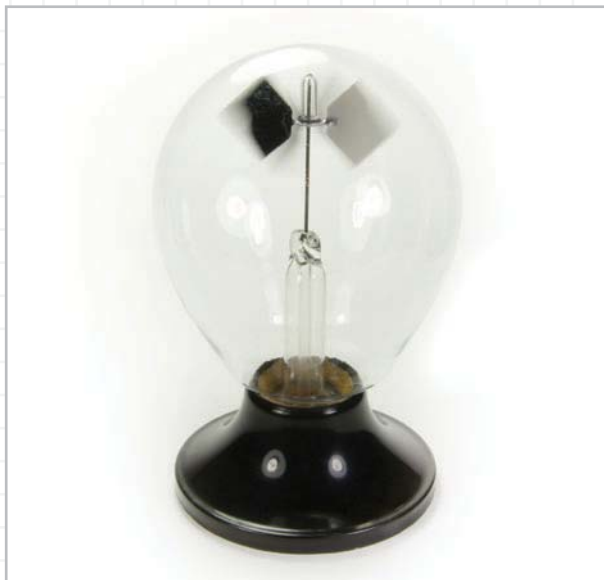
The vanes of a radiometer spin when they are exposed to bright light.
