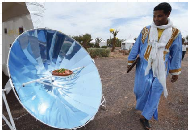
Radiation carries energy from the sun. By using a solar oven, this energy is directed at a single object to cook food.
