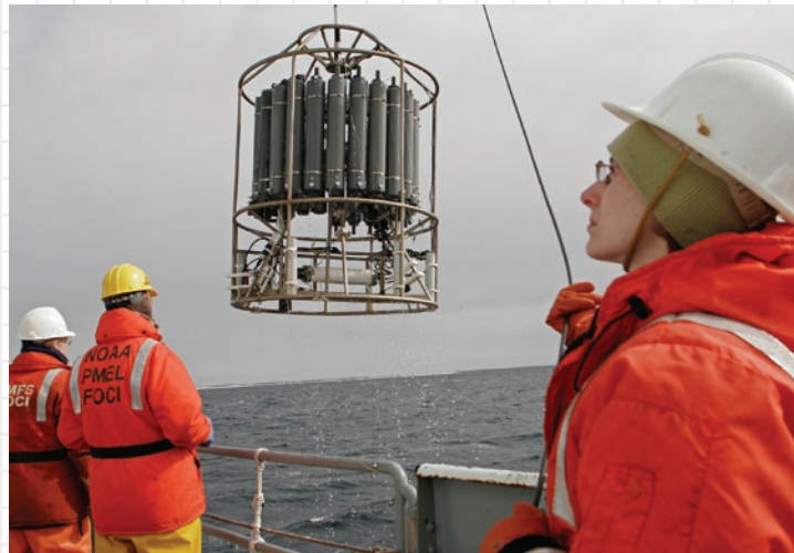
A physical oceanographer brings a CTD instrument onto a research ship. The CTD takes many measurements of conductivity, temperature, and depth.
