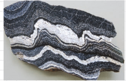
This rock is made up of light and dark bands of minerals that were chemically changed from their original form by intense pressure and temperature.
