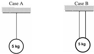
2. Determine tension in each cable. (Hint: There is more than one way to define the system.)
