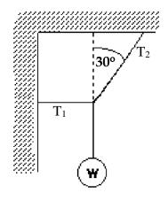
a. Write the equation for the sum of the forces in the x-direction. Solve for the value of  $T_2$ .
